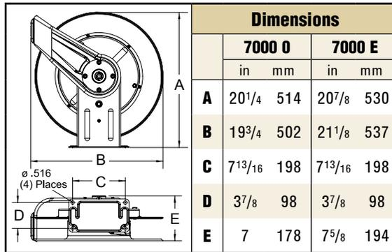
Series 7000 E reels are the same as 7000 O reels except **E Series reels are fully enclosed**. To order, change the model number suffix letter O to E. Example, 7650 OHP becomes 7650 EHP. Add 17 lbs. to open reel weight.
