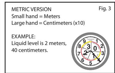
9. Once you have the hands in the correct position, hold the screwdriver firmly in position and tighten the thumb nut on the shaft.
