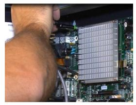
Figure 3-4 Connect Printer USB to Integra Main Board
