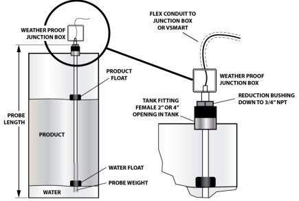
Figure 10-2 Flex Probe Installation Diagram
