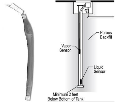
Interstitial Hydrocarbon Liquid Sensor Installation
