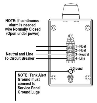
Figure 7-1 Tank Alert Wiring Connections
