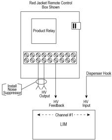
Figure 5-6 Red Jacket Wiring Connections
