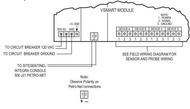
Figure 4-4 VSmart Module Connections
