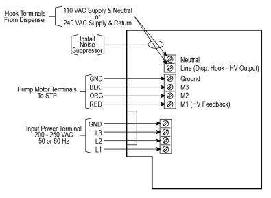
Figure 5-3 FE Petro Wiring for Variable Speed Control
