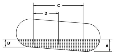
Figure 8-5 Calculating Probe Offset
