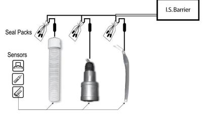
Figure 12-1 Multi-drop Sensor on I.S. Barrier
