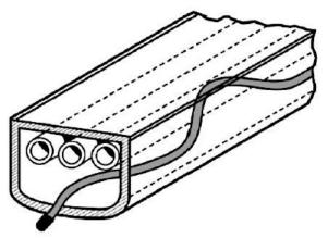
Figure 12-3 Interstitial Sensor Installed in Manway
