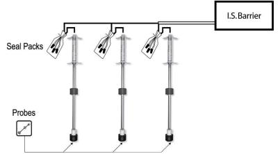
Figure 9-1 Multi-drop Probes on I.S. Barrier
