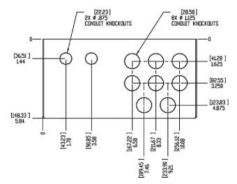
Figure 4-2 VSmart Module Knockouts
