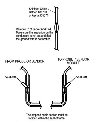
Figure 8-2 Probe-Cable Seal-Offs
