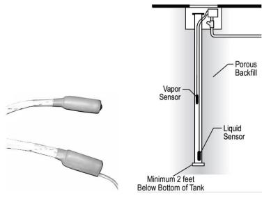
Hydrocarbon Liquid Sensor Installation
