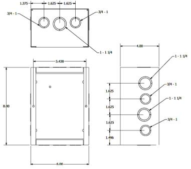
Figure 5-1 LIM Module Dimensions and Knockouts
