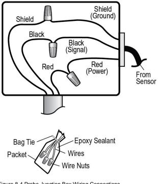
Figure 8-4 Probe Junction Box Wiring Connections
