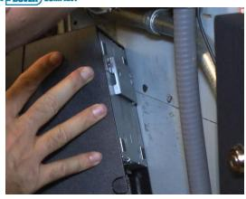
Figure 3-3 Install External Thermal Printer
