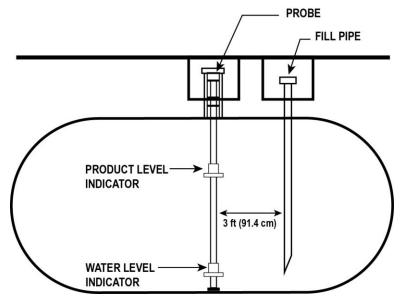
Figure 8-3 Probe Placement
