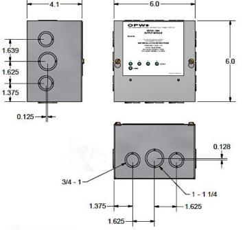
Figure 6-1 OM4 Module Dimensions and Knockouts
