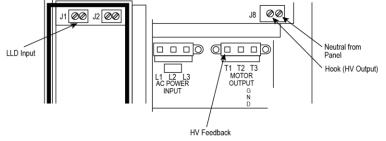
Figure 5-5 Red Jacket Wiring for Variable Speed Control
