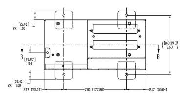
Figure 4-3 VSmart Module Dimensions
