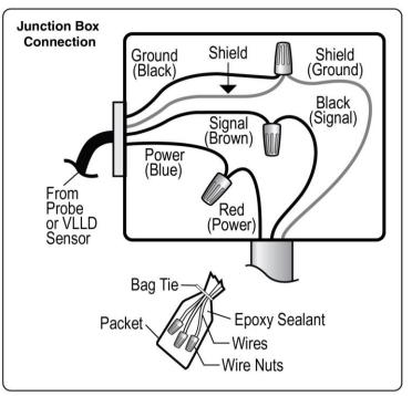
Figure 11-6 VLLD Wiring Connections
