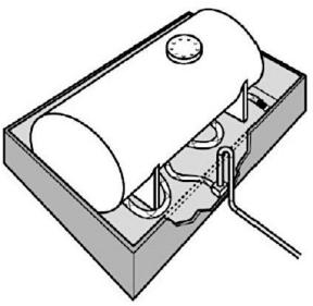
Figure 12-2 Interstitial Sensor Installed in AST
