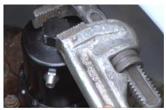
Figure 11-4 Tighten Sensor
