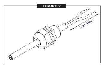
Insert the power cord through the 3/4 inch NPT connection on the side of the electrical box.
