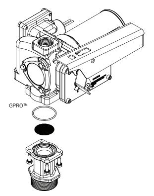
Turn the pump off and disconnect from power. Remove and clean the strainer with a soft-bristled brush and solvent. If the strainer is very dirty, compressed air may be used. If damaged, replace the strainer.
